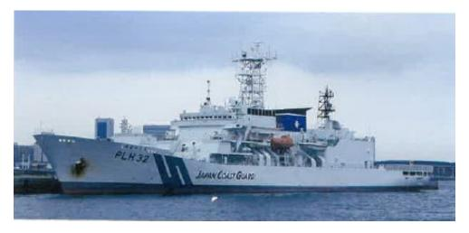
The "Akitsu" is a new helicopter-equipped patrol ship operated by the Japan Coast Guard, which was officially delivered in November 2013. The ship is about 150 meters long and 17 meters wide equipped with two 20mm guns and two 40mm guns. The
