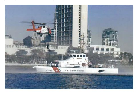
The *Protector*-class (also known as the Ocean Protector-class) entered service in 2002, with a total of 73 built. The boat is 27 meters long, has a displacement of about 92 tons, a speed of 25 knots (46 km/hour), and a self-sustaining capacity of three days. In 2020, the Department of Homeland Security proposed the 2021 budget for the US Coast Guard, in which eight of the *Protector*-class will be retired one after another, and the mission will be taken over by the Sentinel-class.
