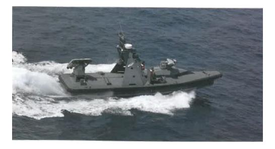
Israel's "Protector" adopts a modular platform design and open structure, which can ideally meet the needs of ship and force protection under various maritime conditions. It has the ability to protect high-value targets, including naval ships, ports, oil facilities, and coastal power plants by providing long-range independent surveillance, identification, and engagement capabilities.
