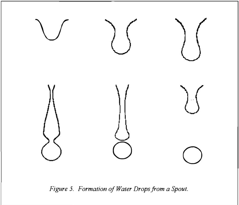
Figure 5. Formation of Water Drops from a Spout.
