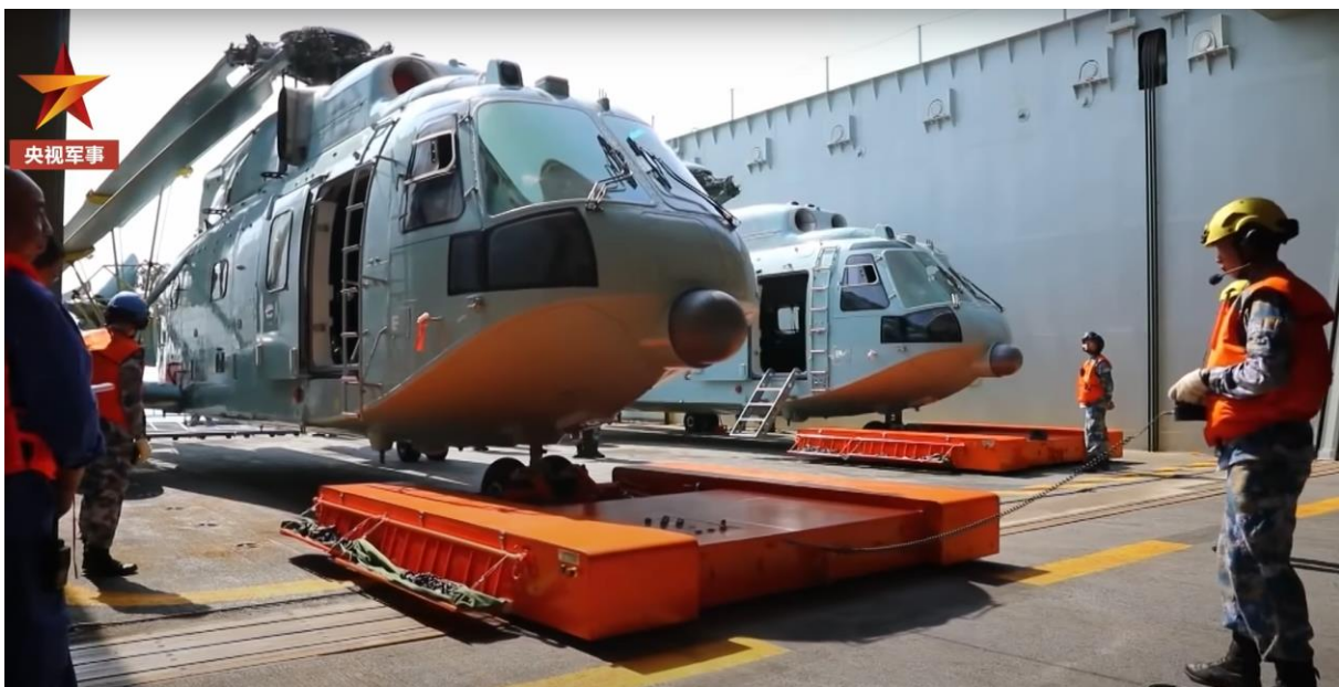
Exhibit 14: Deck crew on the Guangxi train with the PLAN's version of the MANTIS, a low-profile aircraft tug controlled umbilically by the operator to enable aircraft maneuver in confined spaces. 150
