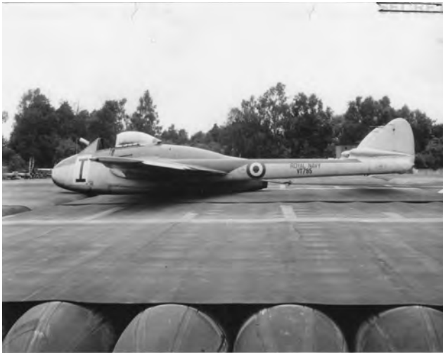
A Fleet Air Arm Vampire on the “flexible rubber carpet” at RAE Farnborough. Note the air-filled “sausages” that support the flexible rubber deck.
