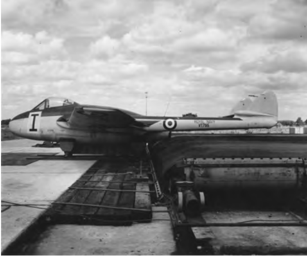
This photo from Farnborough shows how the jet without an undercarriage would be moved off the rubber deck and onto a trolley.
